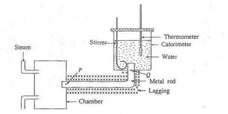
The apparatus shown in the diagram can be used to determine the thermal conductivity of a metal in the form of a rod of uniform cross-section. In this experiment steam at 100 °C is passed through the chamber and the temperature,  $\theta$ , of the water in the calorimeter is measured with time t.
